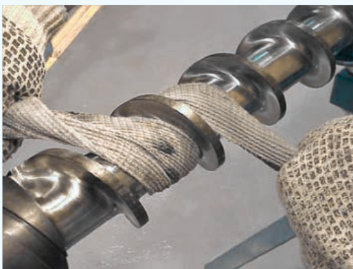
FIG 4 Final cleaning of the screw channels and flight outside diameters returns the screw to its pristine condition.
