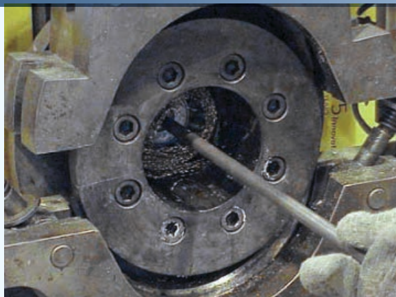
FIG 6 The brush/gauze assembly is pushed into the bore of the barrel. Then an electric drill is used to rotate the assembly until it moves easily throughout the bore.
