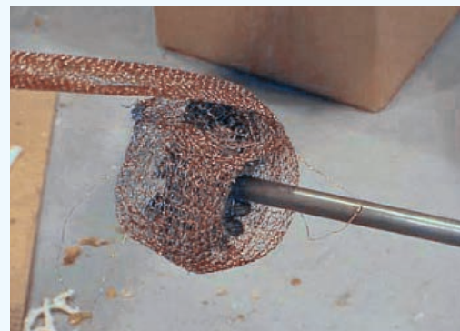
FIG 5 The first step in barrel cleaning is to wrap copper gauze around the outside diameter of a round wire brush at the end of an extension rod.
