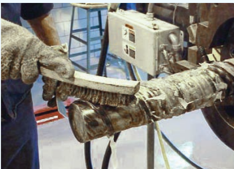
FIG 3 Use a brass wire brush to clean away the purging resins from the screw channels.
