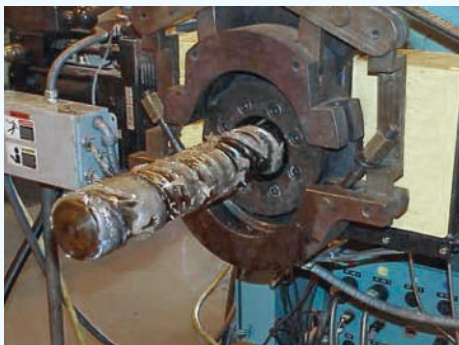
FIG 2 Screw cleaning begins by pushing the screw forward until the first four or five turns are exposed.
