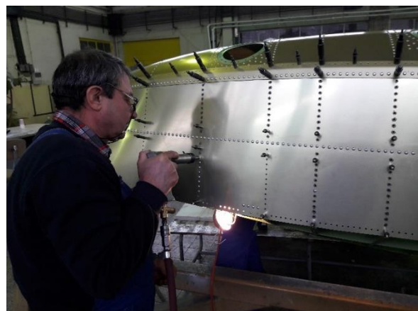
Figure 49: Operator performing riveting on the float
