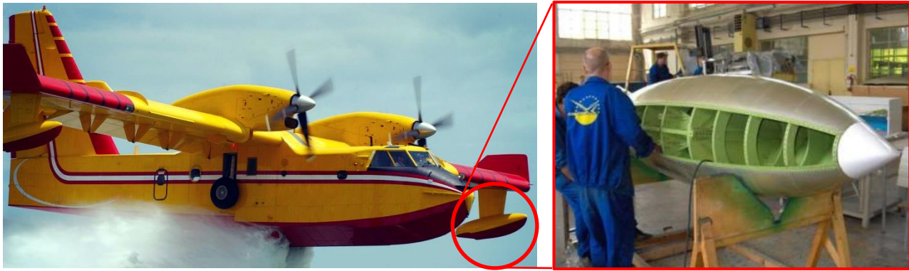
Figure 47: CL-415's float subcomponent - installation and assembly
