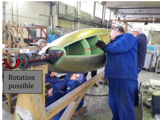
Figure 50: Float installation on its support for riveting
