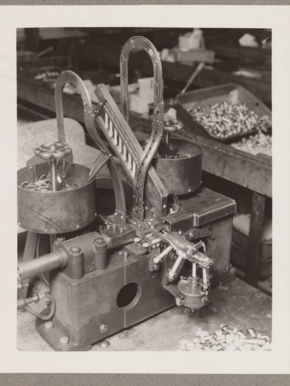
SEMI-AUTOMATIC RELAY SPOOL HEAD ASSEMBLY MACHINE ,
