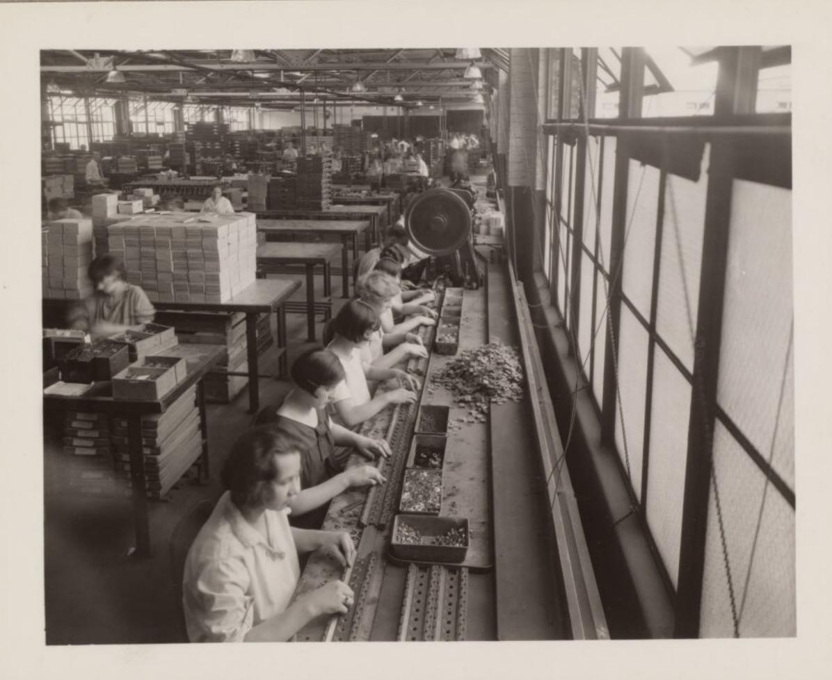
PROGRESSIVE ASSEMBLY OF TRANSMITTER BRIDGE
