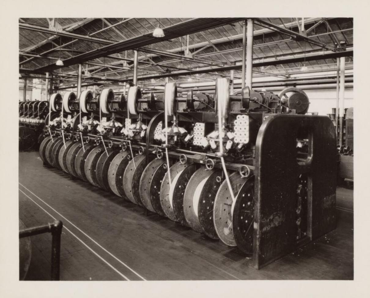
SWITCHBOARD CABLE BRAIDING MACHINES
