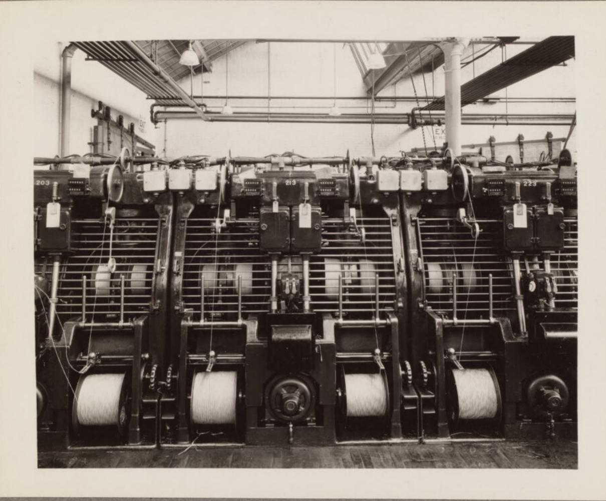
LEAD COVERED CABLE WIRE TWISTING MACHINES
