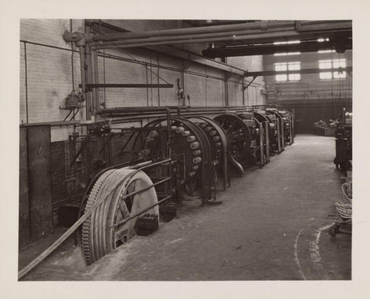
SUBMARINE TELEPHONE CABLE ARMORING MACHINE
