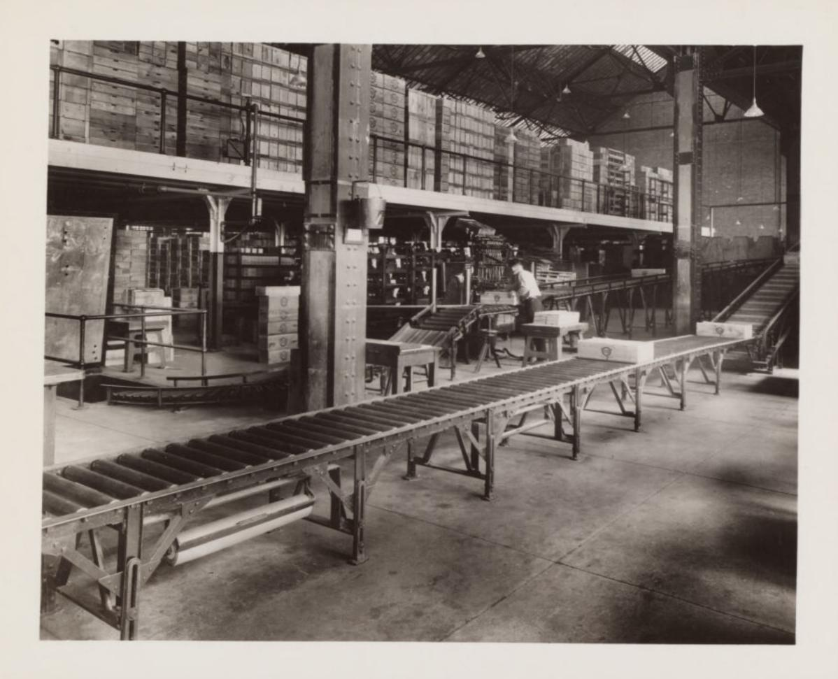
PACKING DEPARTMENT-SHOWING NAILING MACHINE AND CONVEYOR SYSTEM
