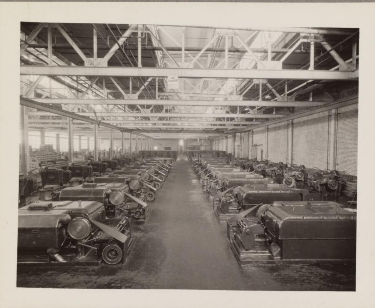
WIRE MILL-HEAVY WIRE DRAWING MACHINES
