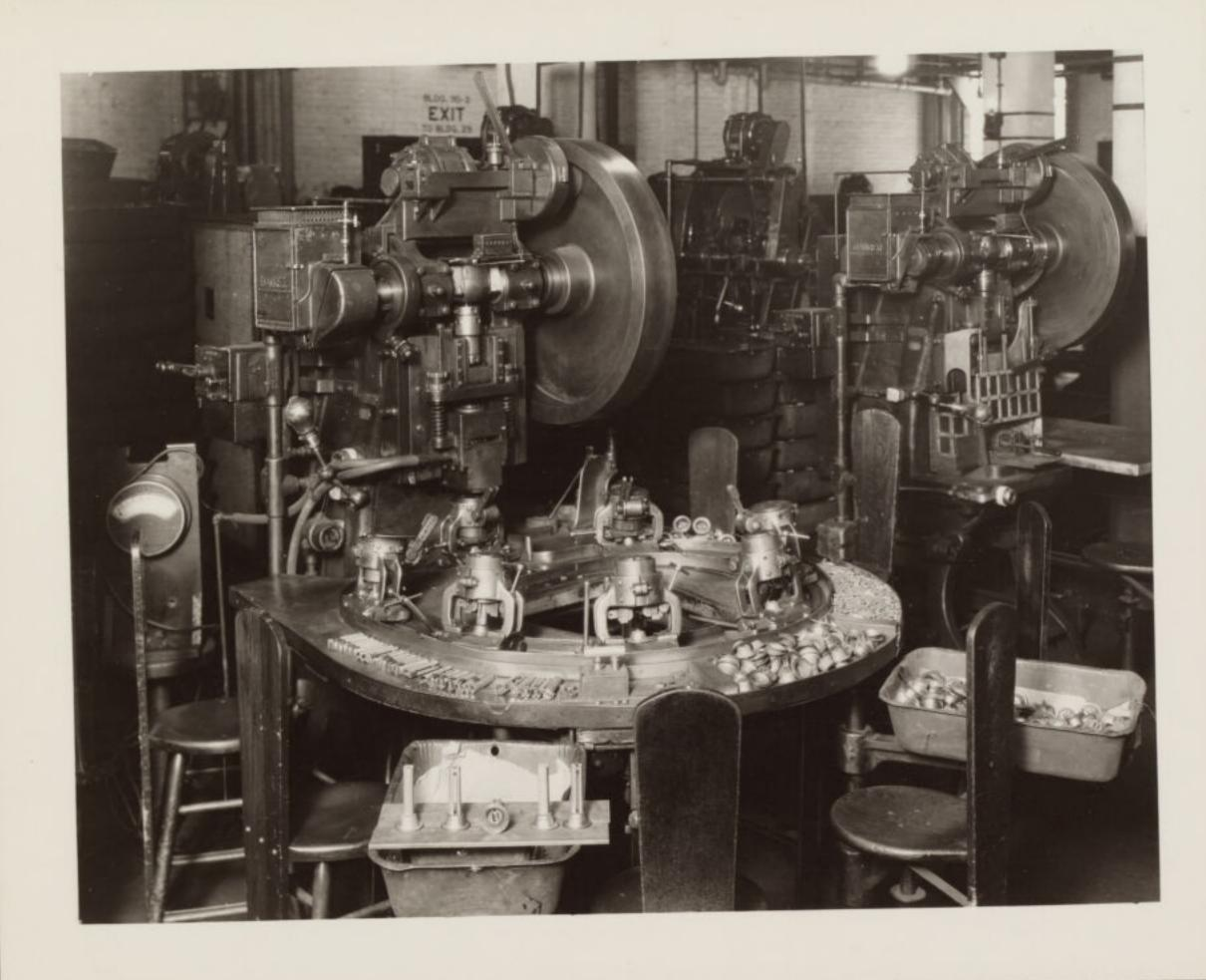
WELDING MACHINE-RECEIVER MAGNET AND CUP ASSEMBLY-SHOWING FIXTURES IN POSITION
