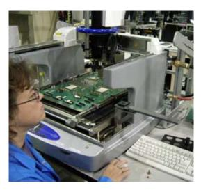
Benchmark Electronics now uses rework equipment designed especially for lead-free assembly.
