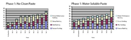
Summary graphs of the print test comparing how well each of the pastes printed onto the test card.
