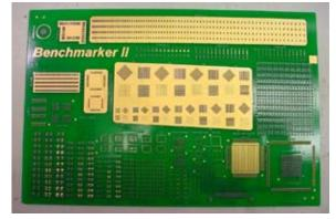
**In-circuit testing (ICT)** determined how well spring-loaded probes could penetrate flux from non-lead solder to make contact with the pads and component leads to test for connectivity. This was performed on circuit boards assembled
