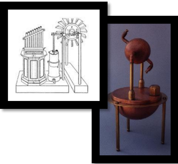
Hero (or Heron) of Alexandria – "aeolipile" – First documented steam engine and a wind organ
