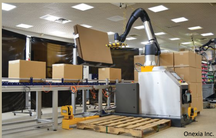
A cobot works in a palletizing cell designed by Onexia.
