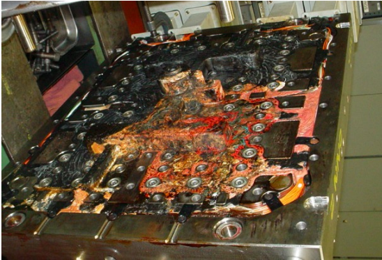
4 Submanifolds / 1 Bridge (57 zones) complete over haul.
