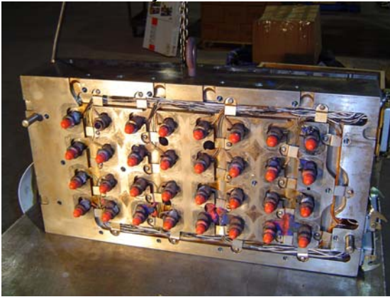
Assembly views after cleaning & components inspection / extrude honing
