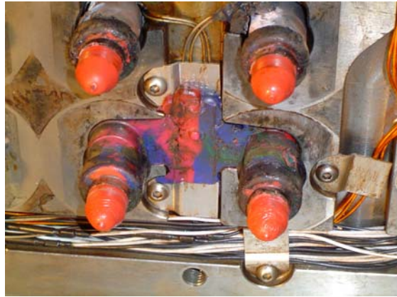
Assembly views after cleaning & components inspection / extrude honing
