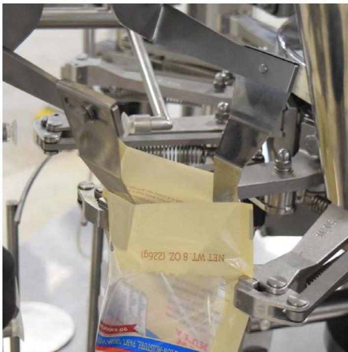
If the bag has a zipper reclosure, a vacuum suction pad opens the lower part of the preformed pouch and opening jaws catch the top side of the bag. The opening jaws separate outward to open the top of the bag and the premade pouch is inflated by an air blower. If the bag does not have a zipper, the vacuum suction pads still open the bottom part of the pouch but only the air blower is engaged.
