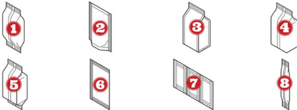
1. **PILLOW BAGS** are the most widely-used and economical packaging format, comprised of two flat panels sealed together on the top and bottom with a vertical seal down the back. This bag type is popular for value-brands, chips, single-serving snacks, and fractional packs of coffee.
