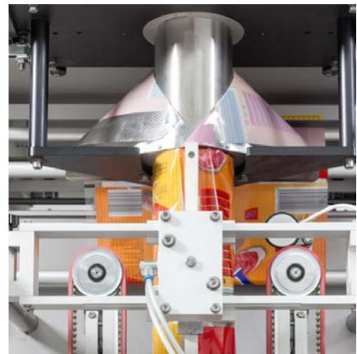
A rotary encoder is placed near the shoulder (collar) of the forming tube. The moving film in contact with the encoder wheel drives it. A pulse is generated for every length of movement, and this is transferred to the PLC (programmable logic controller). The bag length setting is set on the HMI (human machine interface) screen as a number and once this setting is reached the film transport stops (On intermittent motion machines only, continuous motion machines do not stop.)
