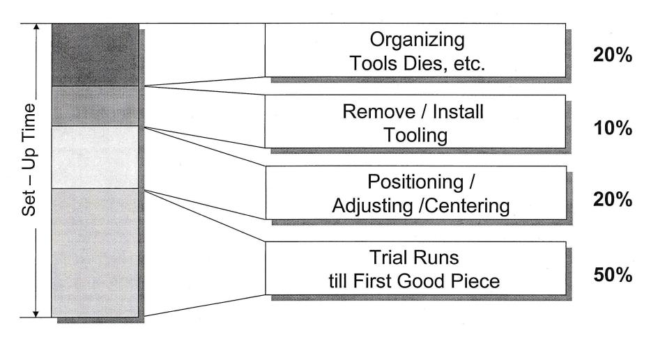
Simple Tools and Techniques can Have a Dramatic Effect on Set-Up Time
