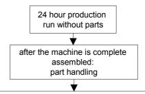
Prepairing for the PCS. manufacture and measure a part. The measurement have to be within the half drawing tolerance. Manufacturing and measuring of the following 5 parts.
