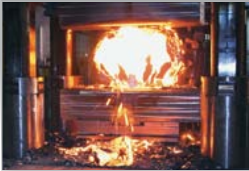
160 t forging grade ingot under the 80/100 MN press
