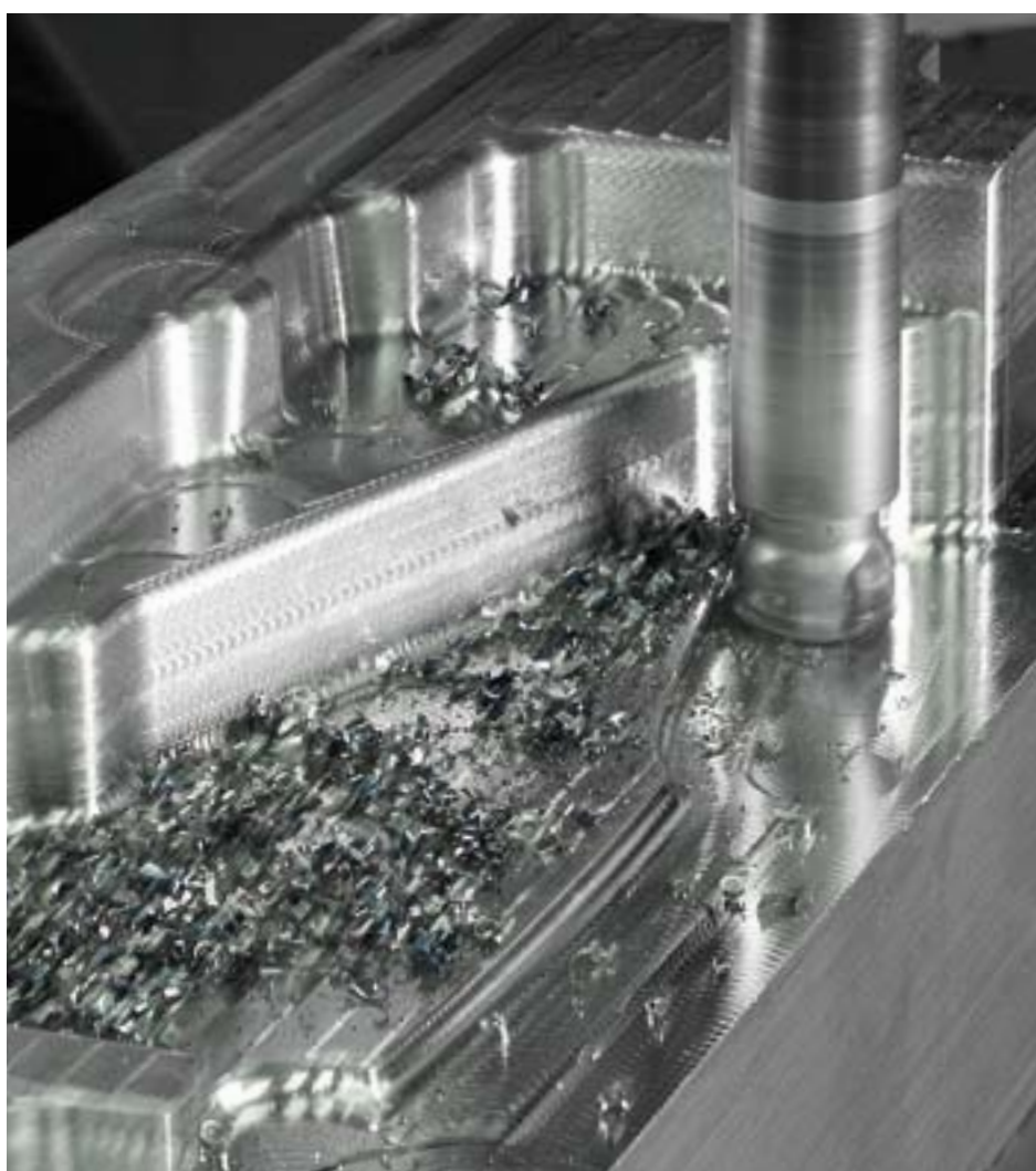
2312 core part undergoing rough machining
