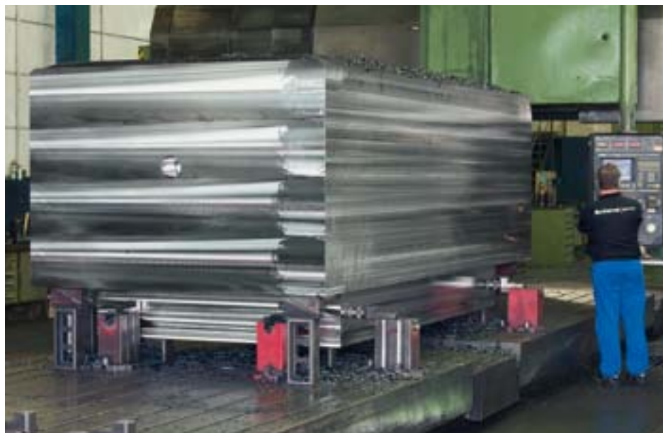
Premachining on gantry milling machines
