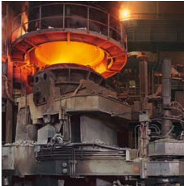
100 tonne ladle furnace (LF-VD/VOD) for producing high-purity tool steels involving secondary and vacuum metallurgical processes
