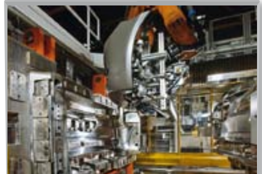
Demoulding the plastic item in production
