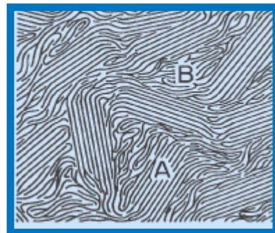
Figure 2. Crystalline (A) and amorphous (B) regions in polyolefin
