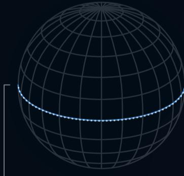
LiDAR emits pulses of infrared light in one or more horizontal planes
