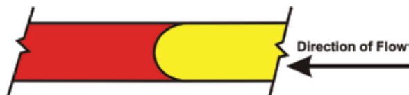
Velocity profile. Material moves faster in the center of a bore.
