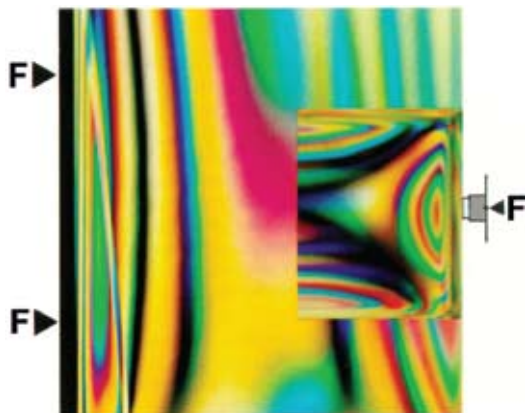
Stress optics photo shows force (F) created during molding.
