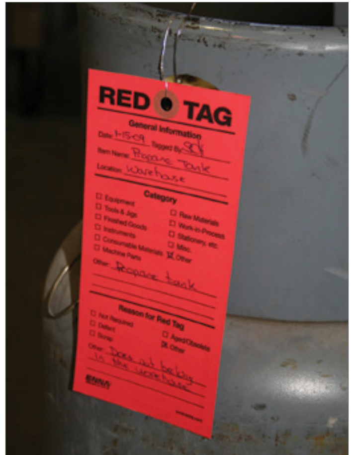
Printed red tags make it easy to identify unnecessary items for removal, tracking, and to provide additional information.
