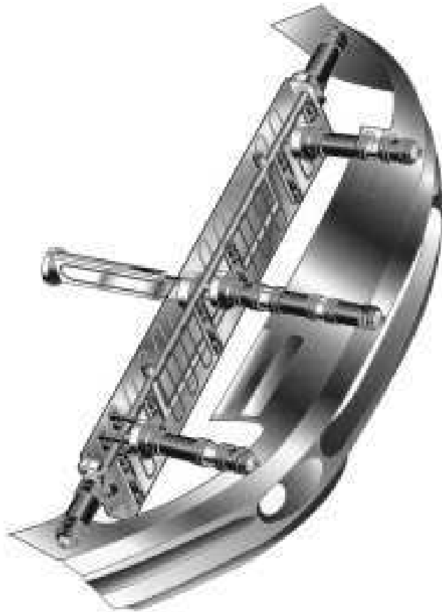
Figure 6.44 Hot runner system for a car fender [6.16].
