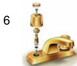
Replaced leaking valve and gasket
