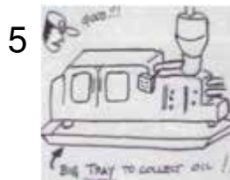
Put a tray to collect oil under the machine
