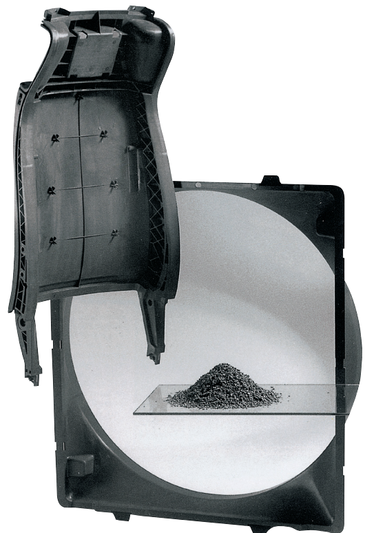
Fig. 18: Engine fan shrouds for buses, made of recyclate obtained from used bus seat backs
